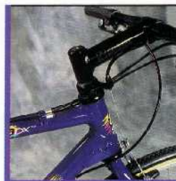
Alpinestars oversize aluminum stem, Easton VariLite tubing.
