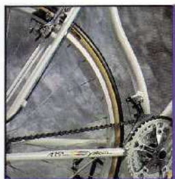
CSS System - 419mm chainstays and curved seat tube provide superior traction and tire clearance.
