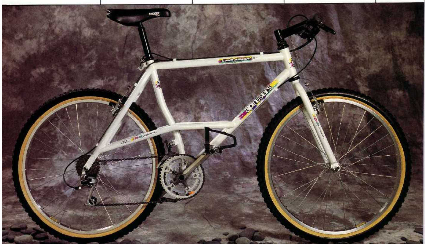
EOS System - Curved seat tube and 403mm elevated chainstays for limitless tire clearance and climbing traction.
