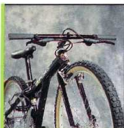
The unique "T-Bike" frame has the lowest standover height of any bike with 26" wheels.
