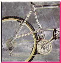
Shimano XTR components with Rapid Fire Plus shifters and 8 speed drivetrain.
