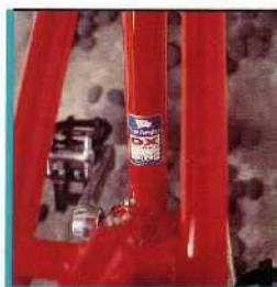
True Temper OXII tubing, specially heat treated to enhance strength and performance.
