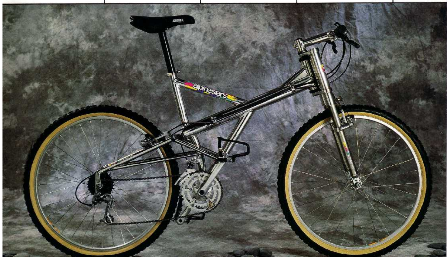
A futuristic frame design that allows a full four inches (100mm) of front and rear shock absorbing travel.
