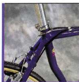
Alpinestars investment cast stainless steel seal collar and cable router.
