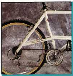
Shimano LX 500 drivetrain with 21 speeds and round alloy chainrings.
