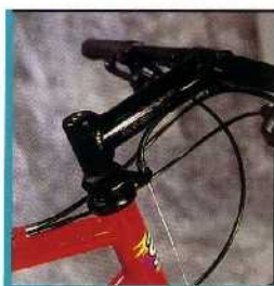
Alpinestars oversize aluminum stem, Easton VariLite tubing.
