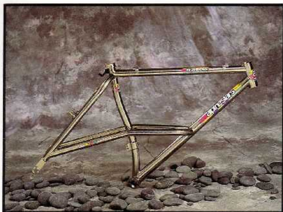
Alpinestars oversized aluminum fork, Easton VariLite tubing. All welded construction.
