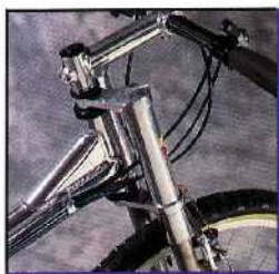
Our rigid upside down triple clamp fork with an Alpinestars braking system provides the front wheel with four inches (100mm) of progressive travel.
