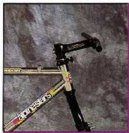
Alpinestars clamp-on stem, Easton VariLite tubing. Tange Superlite headset.
