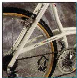
EOS System - Curved seat tube and 403mm elevated chainstays for limitless tire clearance and climbing traction.
