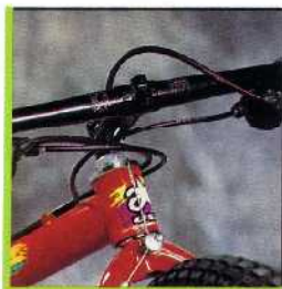
ZSS System - Clamp-on stem, Zero stack headset and special length fork combine to reduce standover height and provide proper riding position.
