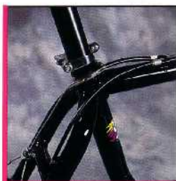
Alpinestars investment cast stainless steel seat collar and cable router.
