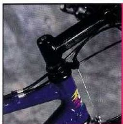
Alpinestars oversized aluminum stem, Easton VariLite tubing.
