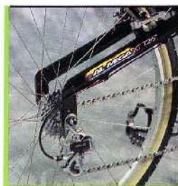
Cold forged rear dropouts are specially designed for our mono rear stays.
