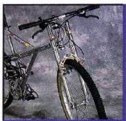
A futuristic frame design that allows a full four inches (100mm) of front and rear shock absorbing travel.
