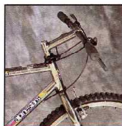
Alpinestars 3-2.5 Titanium oversized stem and Tange Superlite headset.
