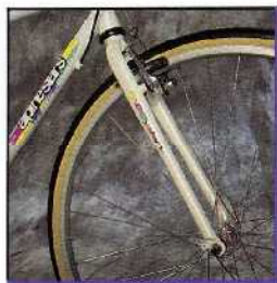
Unicrown fork design with ovalized Cro-Moly blades.
