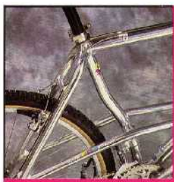
EOS System - Curved seat tube and 403mm elevated chainstays for limitless tire clearance and climbing traction.
