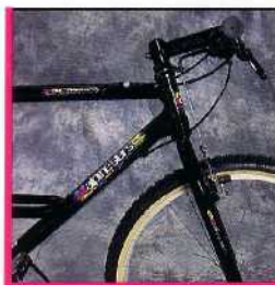
Alpinestars ODS System - 28.6mm 7005 series aluminum handlebars, Easton VariLite aluminum clamp-on stem and Easton VariLite aluminum fork.
